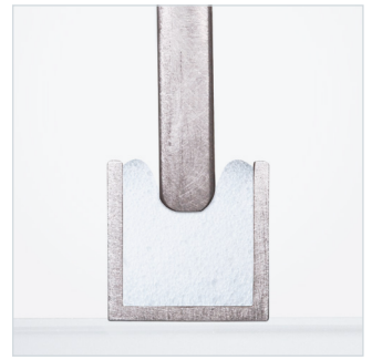
Cross-section of a silicone foam bead in the groove and pressed to approx. 30 %
