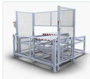
Optional: WT 1-LEVEL shuttle/sliding table with two pick-up plates operating in shuttle mode in one plane
