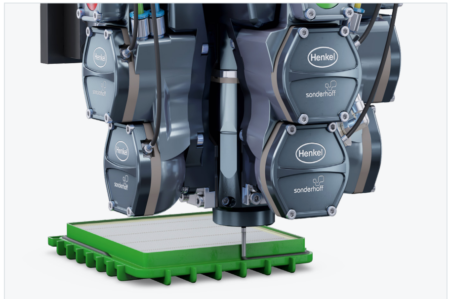
Dosing application of PU foam using a precision mixing head for sealing the filter frames of HEPA filters for vacuum cleaners
