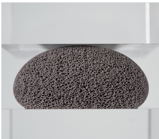
Cross-section of a polyurethane foam bead – uncompressed
