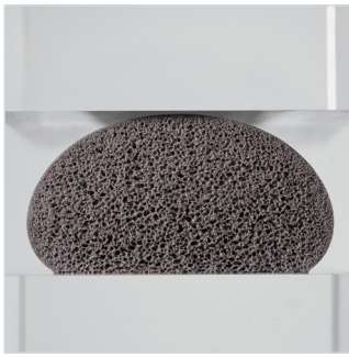
Cross-section of a polyurethane foam bead – uncompressed
