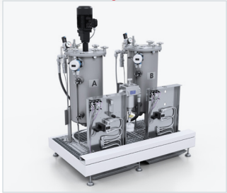
Separately installed material pressure tanks (24 l or 44 l, single-walled or double-walled) with minimum level sensors, on a grating platform with adjustable leveling feet and drip tray
