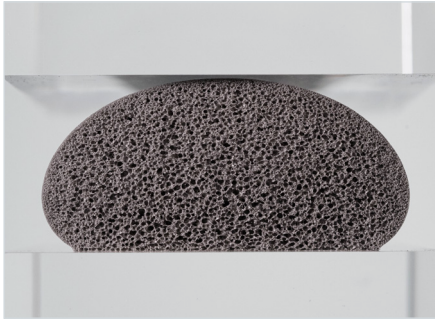
Cross-section of a polyurethane foam bead – unpressed
