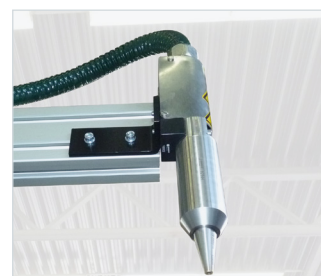
The optional plasma nozzle mounted on the back of the CNC Y-axis applies the plasma in parallel to the seal application onto plastic surfaces of the component in the same contour.
