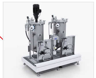
Material pressure tanks (24 l or 44 l, single-walled or double-walled) with minimum level sensors, on a grating platform with adjustable leveling feet and drip tray
