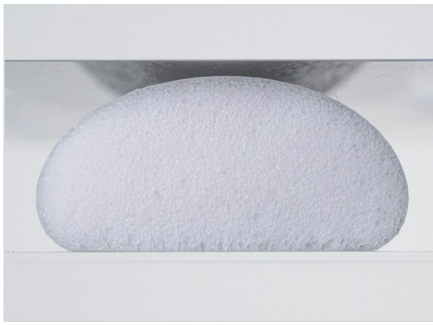
Cross-section of a silicone foam bead – unpressed
