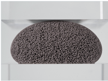
Cross-section of a polyurethane foam bead – unpressed
