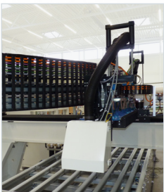
Primer application unit – the optional primer nozzle mounted on the rear of the CNC Y-axis applies the primer in parallel to the seal application on powder-coated or stainless steel surfaces in the same contour.
