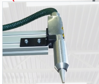
The optional plasma nozzle mounted on the back of the CNC Y-axis applies the plasma in parallel to the seal application on plastic surfaces in the same contour.
