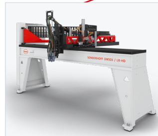
Highly dynamic LR-HD 3-axis linear robot for precise guidance of mixing heads for the application of polymer reaction materials. The rack-and-pinion drive with high stiffness and acceleration enables dynamic application speeds.
