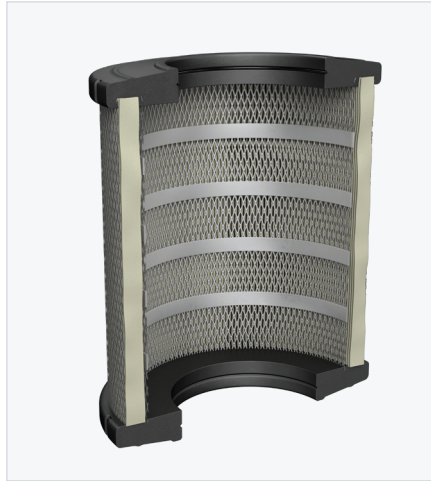
Cross-section of radial air filter showing the connection of filter pack and metal support frame to the PU foam.
