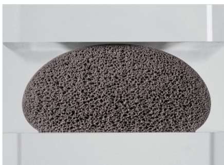
Cross-section of a polyurethane foam bead – uncompressed
