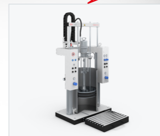
Optional for A- and B-material component: automatic barrel-type pump station for 30 to 200 liter containers, with scoop piston pump, as twin-column lifting unit, for highly viscous / pasty materials
