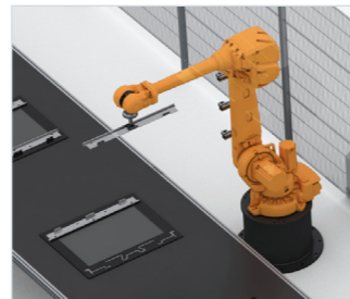
The 6-axis robot joins the metal brackets for attaching a holding frame to the inside of the oven glass door
