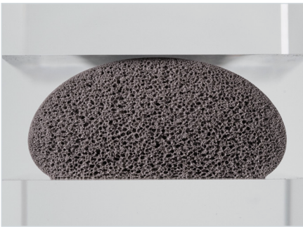
Cross-section of a polyurethane foam bead – unpressed
