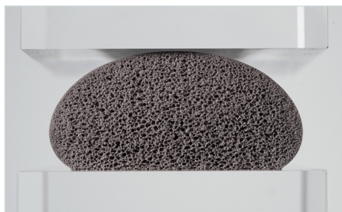
The unpressed polyurethane foam gasket before installation.
