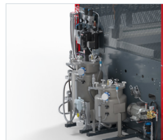
The material pressure tanks have a capacity of 44 l for the A component and 24 l for the B component, thus accommodating the typical asymmetrical mixing ratio.
