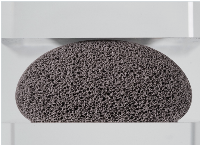
Cross-section of a polyurethane foam bead – unpressed
