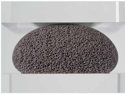
Cross-section of a polyurethane foam bead – unpressed
