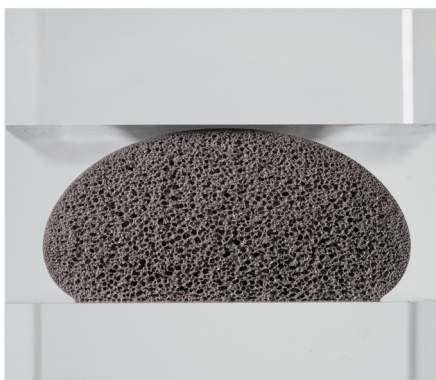
Cross-section of a polyurethane foam bead – unpressed
