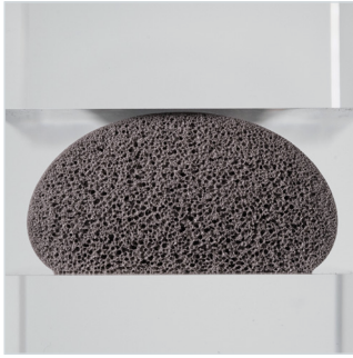
Cross-section of a polyurethane foam bead – uncompressed
