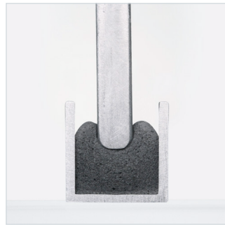
Cross-section of a polyurethane foam bead in the groove and compressed to approx. 50 %
