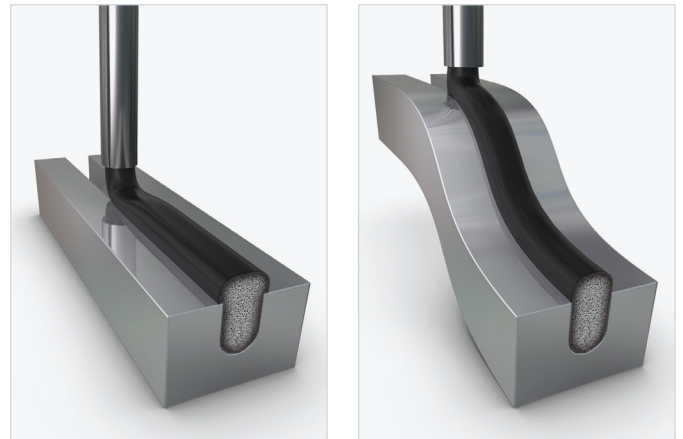
The different reaction phases of the sealing foam in the chronological sequence
