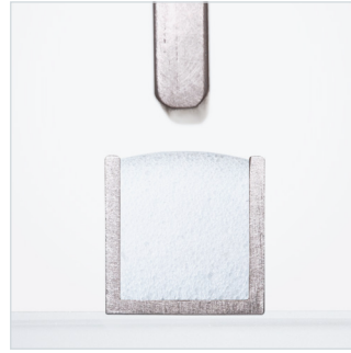
Cross-section of a silicone foam bead in the groove without compression
