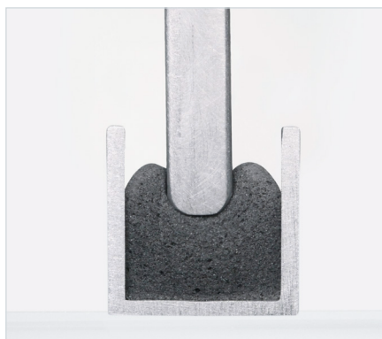
Cross-section of a polyurethane foam bead in the groove and compressed to approx. 50%
