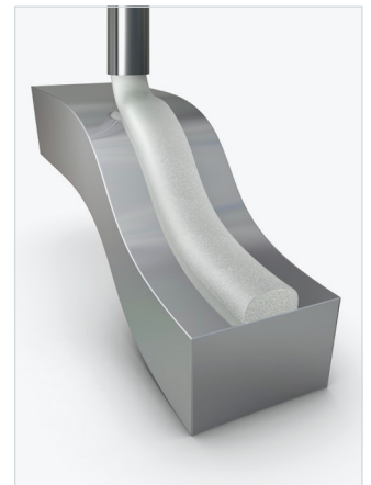
The different reaction phases of the sealing foam in the chronological sequence
