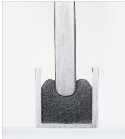
Cross-section of a polyurethane foam bead in the groove with approx. 50% compression
