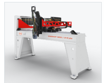
Optional: Highly efficient LR-HE plus 3-axis linear robot for precise guidance of mixing heads for the application of polymer reaction materials. The Omega toothed belt drive enables high application speeds for components with medium and large radii.
