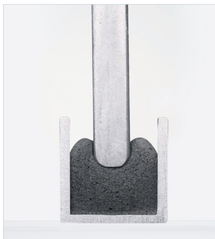
Cross-section of a polyurethane foam bead in the groove and pressed to approx. 50%
